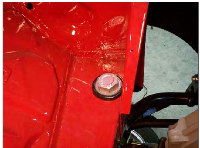
**Step 2:** Drill six holes to support the bottom of the subframe using a 5/16” drill bit. Use the six supplied 5/16” bolts with plates to fasten the subframe to the car on the lower side. The plates will go inside of the car to give the subframe extra support. After the six bolts are in place and tight, tighten the two large subframe mounting bolts on top of the frame. See photos.
