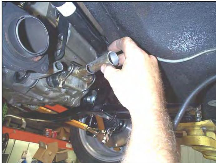
**Step 4:** Reattach lower shifter end (as shown in following photo). The shifter rod reducers will be needed to rebuild the shifter linkage (shifter rod reducers are shown being held in previous and following photos).
