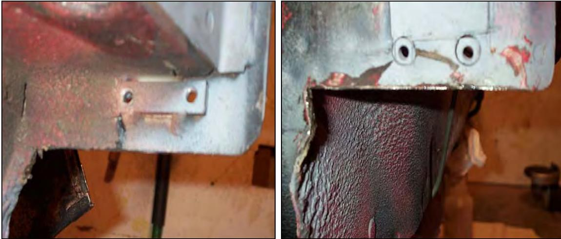
Step 5: Cut out behind grille: You will need to remove any excess metal behind your grille (See Photo below). This will give you maximum flow and cooling ability.
