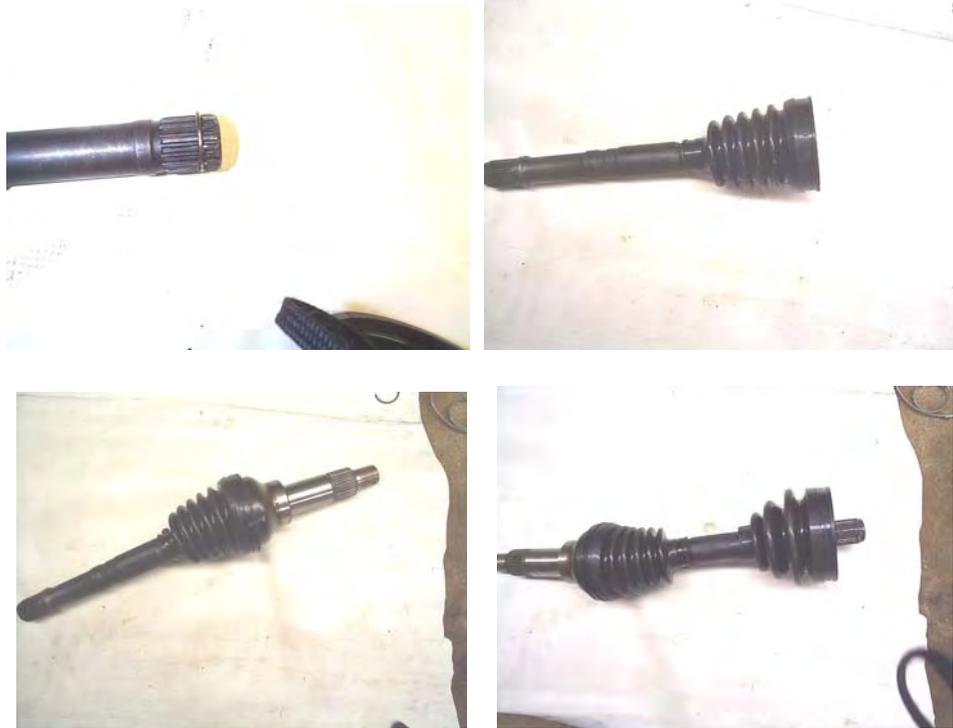
**Honda Axle End Assembly:** Assemble large splinned side of axle with the Honda cv joint assembly. (See following four Photos)
