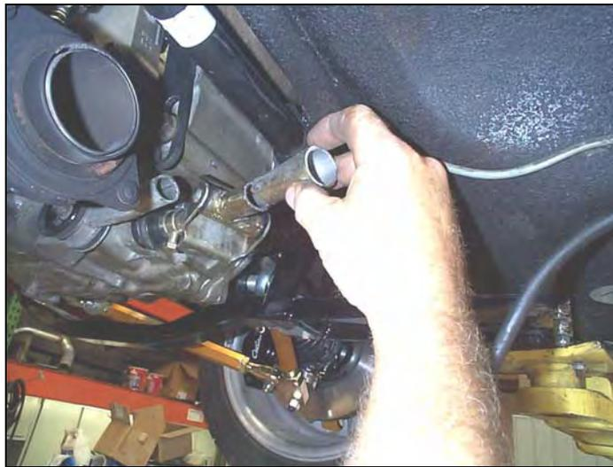
**Step 4:** Reattach lower shifter end (as shown in following photo). The shifter rod reducers will be needed to rebuild the shifter linkage (shifter rod reducers are shown being held in previous and following photos).
