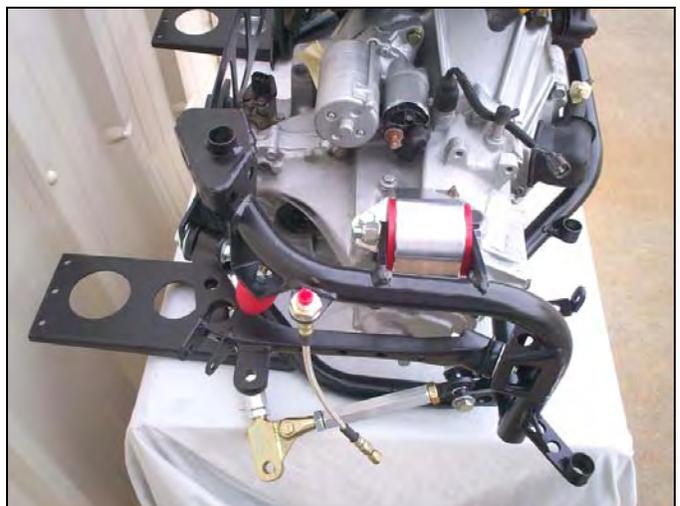
**Step 3:** Attach upper bump stops. Mini bump stops with the single stud will work here.
