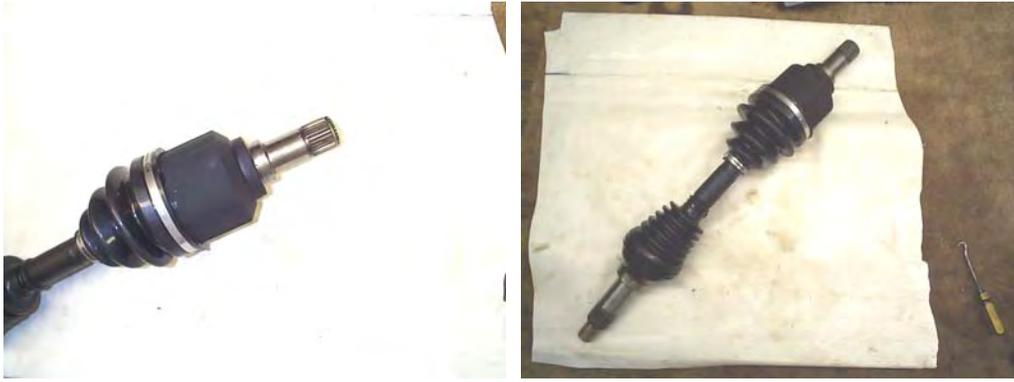
**Axle Installation:** Simply slide one of the axles into the transmission and the other into the engine mid-shaft until the axles lock into place.
