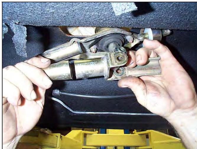
**Step 5:** Rebuild the shifter linkage using ¾” metal pipe. Bend and weld pipes so that all gears can be easily shifted to and from without hitting the body or anything else. (See following photo)
