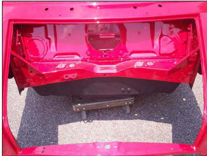
**Step 2:** Remove inner fenders: Cut and remove both inner fenders as shown. You will need this extra space for the width of the subframe.
