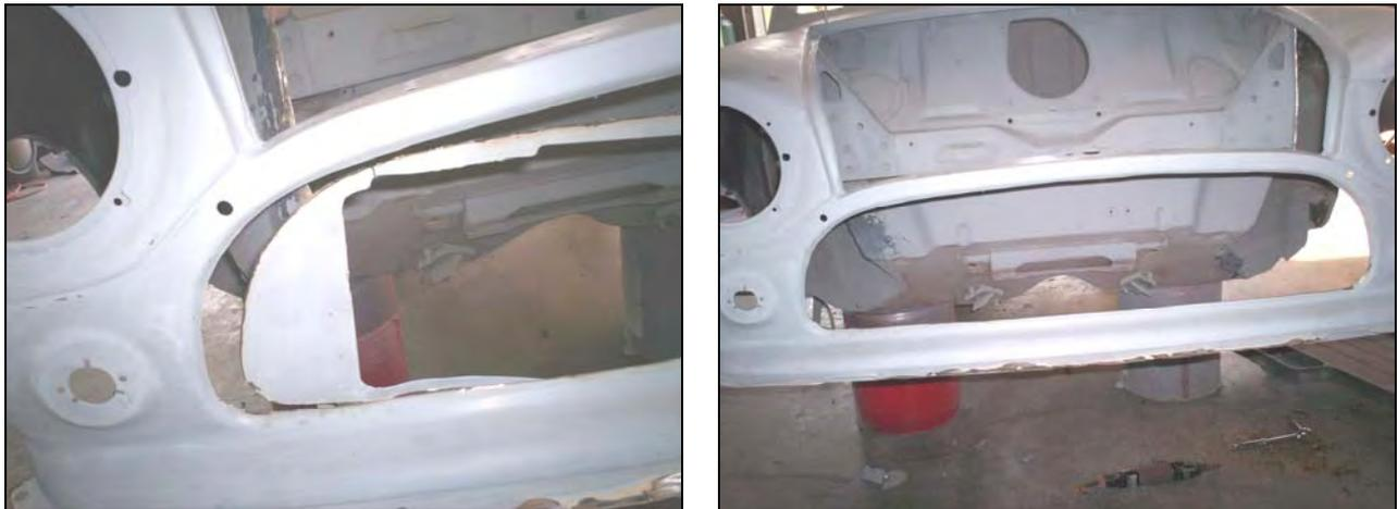
Step 6: Remove all inner metal bracketry that is attached to the lower valence. Cut off lower front valence 1" below bumper lip at intersection. At this point you will need to reattach and weld valence to leading edge of bumper lip as shown.
