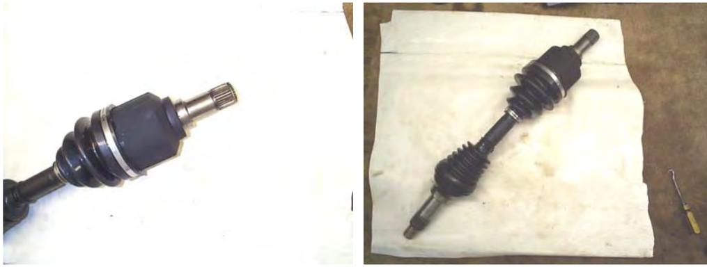
**Axle Installation:** Simply slide one of the axles into the transmission and the other into the engine mid-shaft until the axles lock into place.
