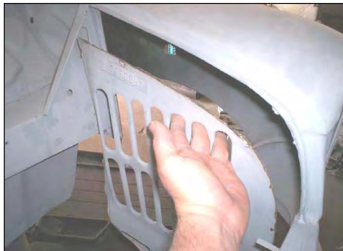
Step 3: Cut out metal just below stock shock mount. This is needed to fit the MTD subframe (See following two photos).
