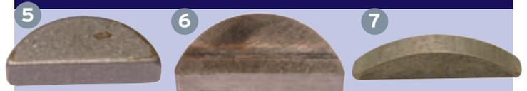
To aid accurate timing when using non adjustable timing gear systems, there is a range of proper CNC machined offset cam keys available. These come in 1° increments up to 9°. One tooth round on the gear represents 13° of cam timing, so if you are more than 9° out move the cam gear one tooth in the required direction and use the keys the other way round as they are bi-directional. They are available individually.
