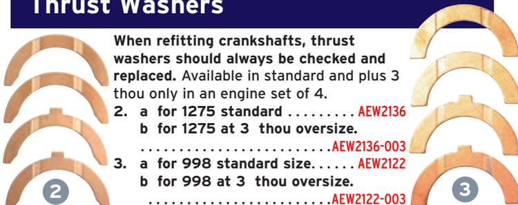
When refitting crankshafts, thrust washers should always be checked and replaced. Available in standard and plus 3 thou only in an engine set of 4.
