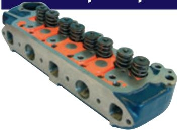
Unleaded with manganese bronze guides and race specEN21 4N stainless steel heat treated valves to eradicate wear.
