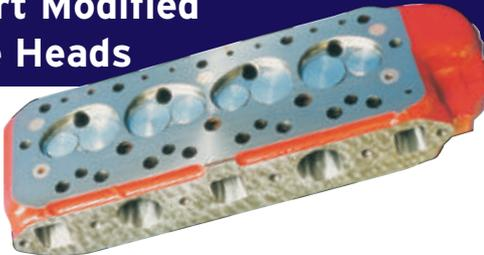
7. 35.7mm inlet valve and 29.2mm exhaust valve with bypass hose pre 1992 . . . . .C-AHT135
