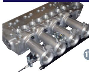
17. Bespoke kit designed to compliment the 8 Port head and optimise its full performance potential. The throttle bodies are a direct body to head design that will fit under the standard bonnet of the mini but for those customers who wish to extend the induction system length, parts will be available to do so.
