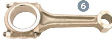
Fitted with ARP nuts and bolts. These are made in a higher grade material and to specific tolerances, including the thread grade. Poor threads vastly reduce torque accuracy causing premature bolt failure.
