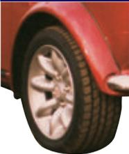
3. The last Rover arches, as fitted to the Sportspack Mini from 1997. Made in rubber and stick out 3 1/2". The bodyline has to be cut away to fit. Finished in correct rubber primer.
