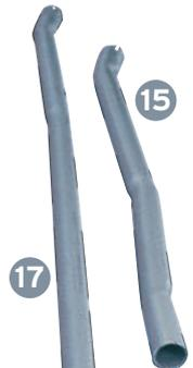
16. Twin box only RC40 performance system which does not include pipe item 14, was designed specifically for Minis by computer and flow bench tested for maximum efficiency and economy, also tested and epitomised in Vizard's 'A' series tuning books. No power loss in engines up to 125 bhp. 1.75" pipe size with internal diameter of 1.625" but entrance hole is flared to 1.75" internal to take item number 14. .... RC40
