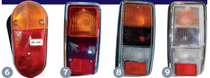
Replacement rear lamps - complete with lenses, back plate, gasket and bulbs.
