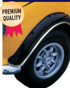
In Fiberglass This arch kit sticks out 2 1/2", including lip, when bodylines (wheel arch and moulding lip) are kept original. Screws are visible and plastic wheel arch moulding can be retained. Rear arch stops at bumper seam line. These are original ST works car copies .....
