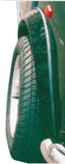
This design of Wide Profile fiberglass arch sticks out 2 1/4" maximum when bodyline (wheel arch and moulding lip) are kept original. Screws are not visible. Front arches taper away at front exposing tire tread. Rear arches stop at bumper seam line. Includes correct body to arch rubber seal. 2 1/4" Upgraded Premium Arches
