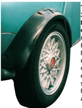
This arch kit sticks out 3" and is used when bodyline is cut away or retained. Originally made as Group 5 Race arch where no body modifications were required, it has become a cheap 'Jack of all Trades' especially when large odd size wheels are used. Rear arches stop at bumper seam line. Widest part at front approximately 5" MS128
