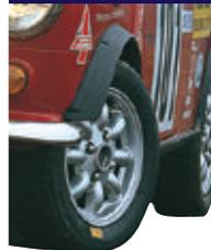
Mini Special Arches. Includes sill trim moulding between arches. This arch kit sticks out 1 3/4" when bodyline (wheel arch and moulding seam) are kept original. Originally fitted to Innocenti Minis and became standard equipment on all Minis from 1984. Screws are visible and rear arch extends beyond bumper seam line. These black plastic arches were originally known as Mini Special Arches. .... GAW117
