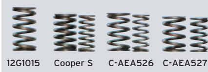
Shows spring heights showing less coils on anti coil bind springs which help eradicate spring crush on high lift camshafts.
