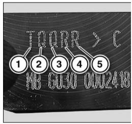
Bearing classification on crankcase upper and lower sections:
