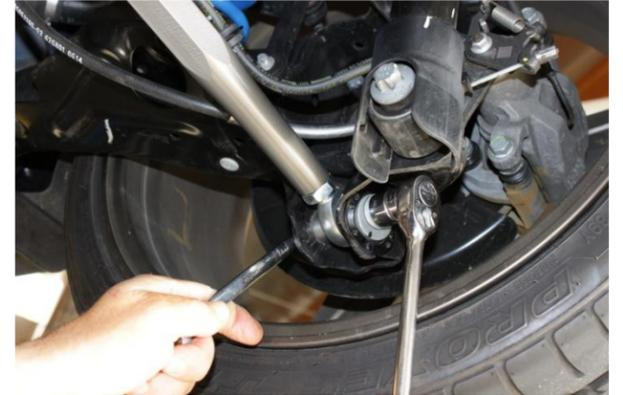
9. Now install outer NM Control Arm to trailing arm using factory bolt and adjusting plate. Line-up previous made pen mark before tightening. Torque to 100Nm (74ft.lbs).
