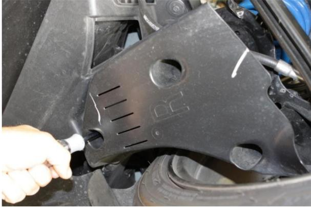
2. Remove the (3) 8mm hex screws retaining trailing arm splash guard.
