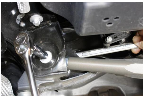
8. Install and tighten NM Control Arm into inner sub-frame mount using original bolt and nut. Torque to 100Nm (74ft.lbs).
