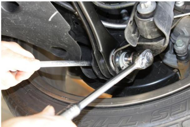
4. Unbolt and remove outer control arm adjusting bolt. Hold bolt head with E14 Torx or 11mm box end wrench and turn nut with 18mm socket.
