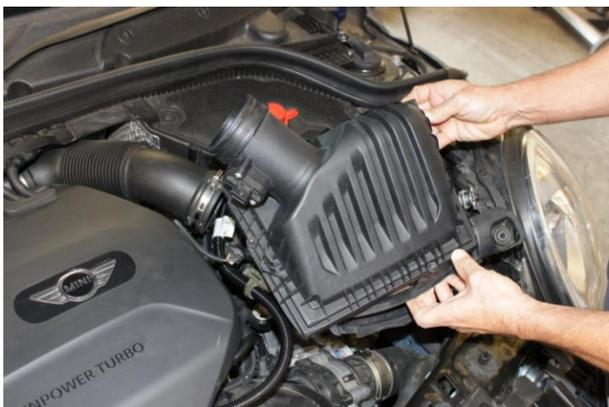
5. Remove the 10mm hex bolt located on driver side of air filter box then lift off. **NOTE:** There are [2] pin mounts that sit into rubber grommets on bottom back side, so a little effort may be required to lift air filter box off rubber mounts.
