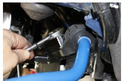
Install original bushing clamps and bolts. Torque to 34 Nm (25 ft-lbs).
