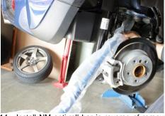
Install NM anti-roll bar in reverse of removal of original bar being careful around brake lines. HINT: Leave plastic wrap on bar to protect finish of bar during installation through sub-frame then remove.
