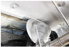
Unbolt [1] 10mm hex nut from exhaust heat shield that connects from sub-frame to unibody.
