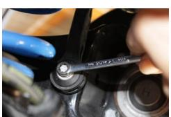
5. Back out lower end-link mounting bolt about a ½" using an E10 Torx or 5/16" wrench or socket. Pull down on anti-roll bar arm due to bushing pre-load and then pull out upper end-link stud from bar. Repeat for other side.
