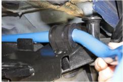
Apply supplied grease to inside of supplied urethane bushings and install on NM anti-roll bar.
