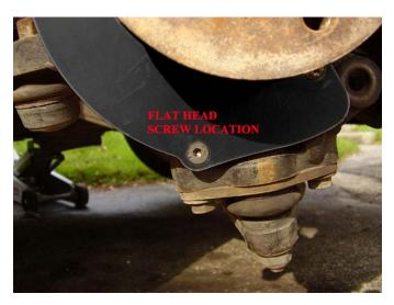
7. Install the scoop on the lower control arm. One method is to position the scoop on the underneath of the control arm and LOOSELY secure it with the supplied tie wraps. (You may need to reposition later.)
