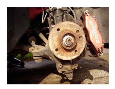
5. The new backing plate can now be installed on the spindle by using (3) of the original Torx style screws, and (1) flat head style screw provided in the kit. When satisfied with the fit, the bolts can then be tightened to factory specs.
