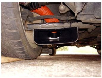
Install the hose between the scoop and the backing plate securing at both ends with the supplied hose clamps.
