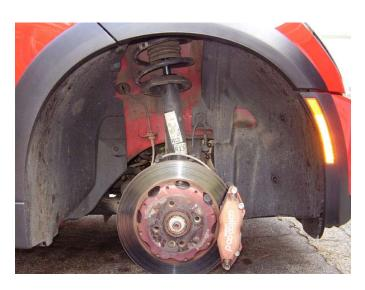
2. Remove the brake calipers by removing the two bolts that secure the calipers to the strut and support them in a way not to damage the brake lines.
