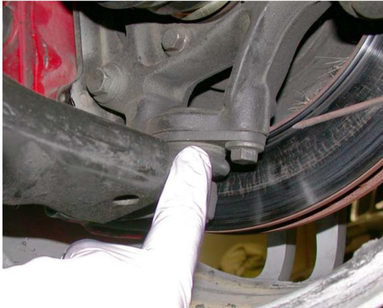
4. Remove the two bolts holding the ball joint to the suspension carrier.
