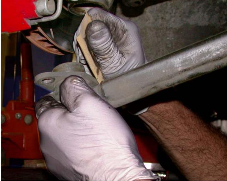
7. Insert the PSA with the flange side up so that it fits snugly into the steering knuckle.
