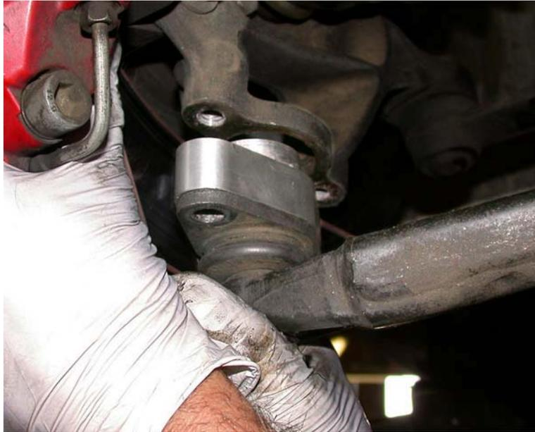
8. Put some Locktite on the bolt threads and secure the PSA with the 16 mm socket.
