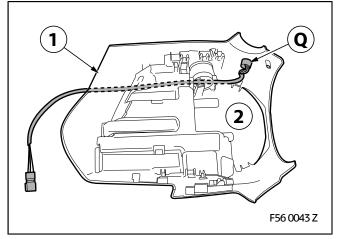
Route the cable from button  ${\bf Q}$  below the foam insert of the steering column trim lower section (1).
