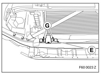
The oval holes in brackets **E** and **F** must point outwards.
