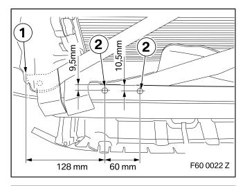
Mark and centre punch the drilling points (2) on the front bumper trim bracket using the dimension shown, starting from the outermost corner of the reinforcing strut (1).
