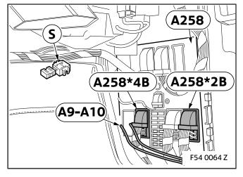
Connect branch A9, GR cable, with miniature connector S to the cable from PIN 4 of plug A258\*4B on the BDC A258.
