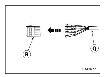
Connect the branches of button  ${\bf Q}$  as follows to socket casing  ${\bf R}$ :
