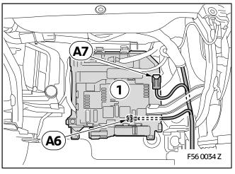
Route branches A1-A5 from the footwell on the passenger side into the engine they and pull through the rubber grommet (1) (use draw-in tool).
