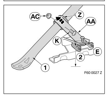
Turn the pipe clip **Z** (see direction indicated by arrow) so that the connecting strut **AA** is stressed and secure it to the reinforcing strut (1) with the screw **K** and nut **AC**.
