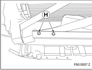
Insert rivet nuts **H** into the holes.
