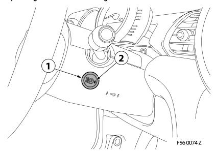
Once activated, the additional headlights light up automatically when the headlights or headlight flash are switched on. Whenever you turn the ignition off/on, you must re-activate the additional headlights.
