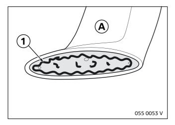
Apply a bead of Betalink 2K glue on the undersurface (1) of the roof spoiler **A** inside the area treated previously with Betalink Primer.
