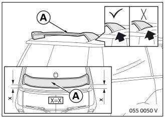
The roof spoiler **A** is positioned via the gap path between the roof and the spoiler.
