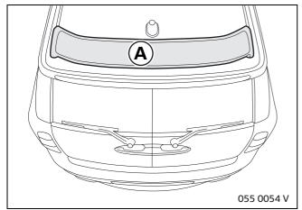
Position the roof spoiler **A** inside the drawn-on outlines, align correctly and press firmly into place.
