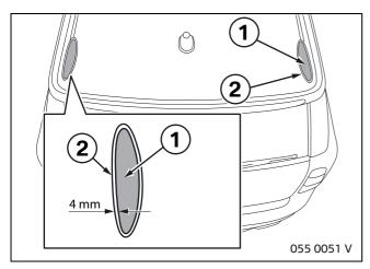
Apply Betalink Primer inside the area marked in grey (1). Leave a gap of approx. 4 mm from the outer edge (2).
