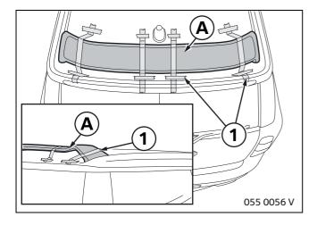
Fix the roof spoiler A in place with adhesive tape (1).
