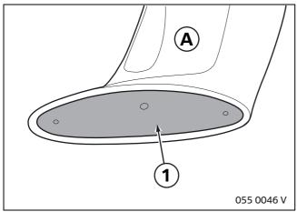
Carefully roughen the undersurface (1) using the sandpaper enclosed with the Betalink 2K glue pack **B** and then clean thoroughly with Betalink Cleaner.
