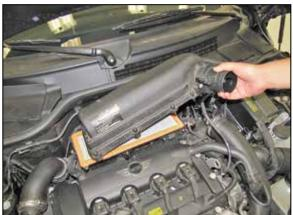
6. Disconnect the intake hose and then remove the upper air box housing assembly and air filter from the vehicle.
