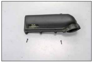
10. Remove two of the factory air filter housing screws from the upper air box.
