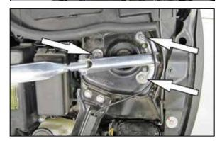
2. Remove the six nuts that secure the strut tower brace to the vehicle struts and then remove the strut tower brace from the vehicle.
