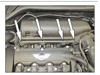
5. Loosen the four screws securing the upper air box housing to the lower housing.
