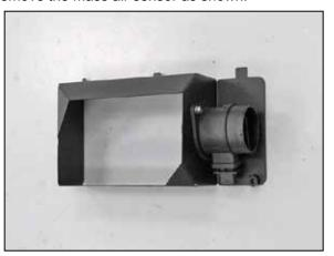
8. Remove the O-ring from the mass air sensor and then secure the mass air sensor to the provided heat shield using the hardware provided.
