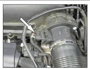
3. Disconnect the mass air sensor electrical connection.
