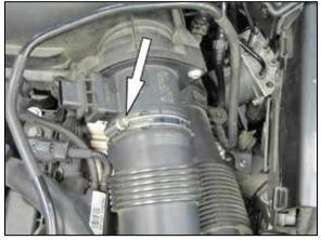
4. Loosen the hose clamp that secures the factory intake hose to the mass air sensor housing.
