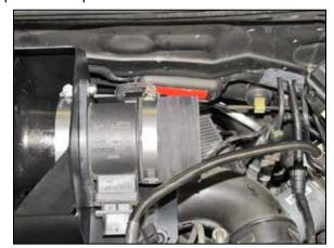
12. Install the provided hose (08440) onto the mass air sensor and secure with the provided hose clamp.
