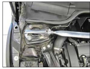
15. Reinstall the strut tower brace and secure with the factory hardware.
