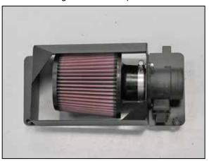
9. Install the K&N® air filter onto the mass air sensor and secure with the provided hose clamp.
