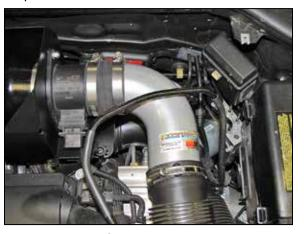
13. Install the K&N® intake tube into the factory intake hose and then into the hose at the mass air sensor. Secure the intake tube with the factory and provided hose clamp.
