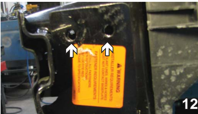
12. Using the baseplate as a template, drill two holes on the side. Do this on both sides using a 13/32" drill bit.
