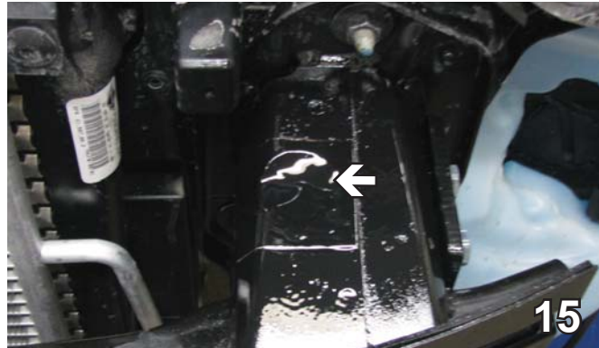
15. Cover the 1 1/4" hole used to install the nut plates with tape and paint black. Do this on both sides.
