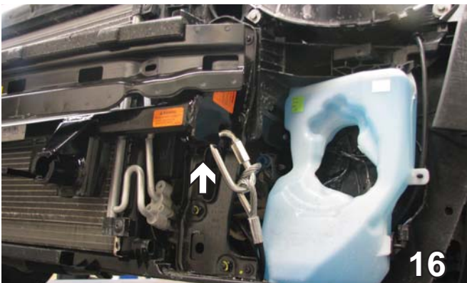
16. The photo above shows recommended installation of the cables to frame of vehicle. If vehicle has additional options (not shown above) which interfere with mounting permanent baseplate safety cables, secure the cables to a solid piece of the vehicle frame as described in instructions included with the permanent baseplate safety cables.
