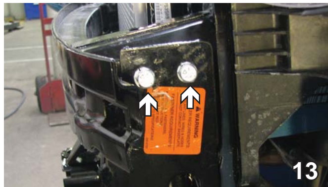
13. Into the holes drilled in the side also insert 3/8-16 x 1 1/4" bolts with Loctite, 3/8" lock washers and 3/8" nut plates. Do this on both sides.
