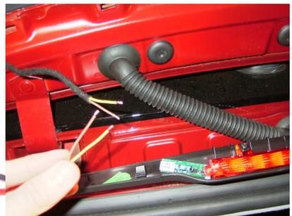
5. With the wires connected insert the plug back into the light and insert pulsar into the panel next to the light, as show in the picture to the right. Reinsert the harness into the wire clips.
