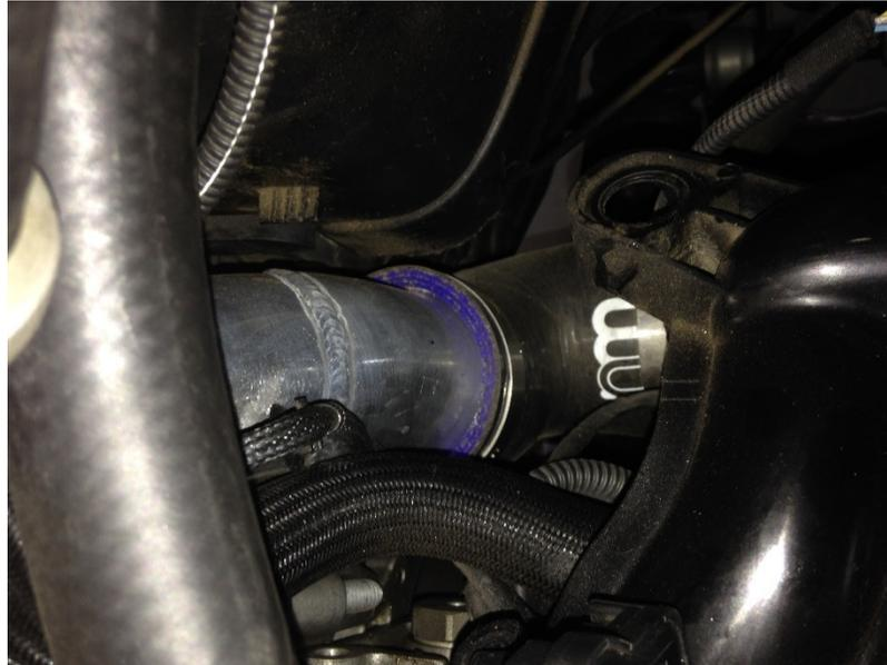
**Figure 10 Intake Manifold Elbow**
