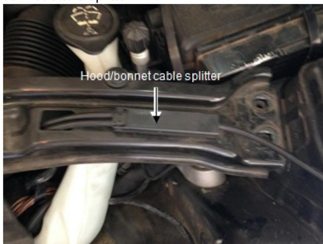
**Figure 6 Cable Splitter Box**
