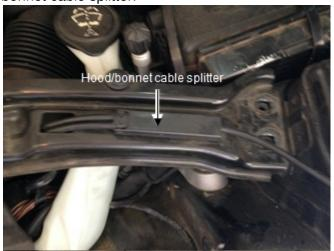
Figure 6 Cable Splitter Box
