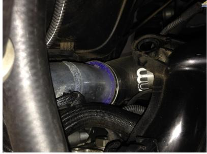
Figure 10 Intake Manifold Elbow
