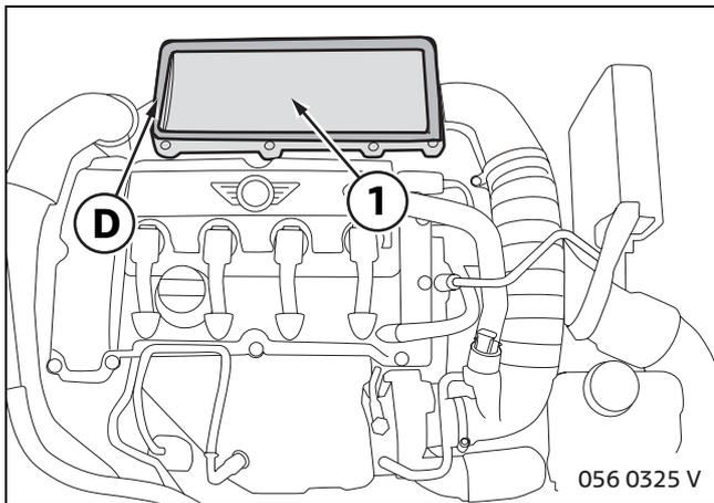
Fit seal **D** on bottom section of air filter housing (1).
