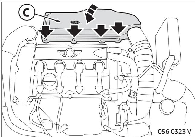
Fit air filter **C** on bottom of housing and secure as per TIS No. 13 71 000.
