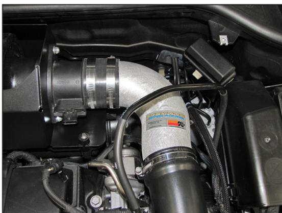
13. Install the K&N® intake tube into the factory intake hose and then into the silicone hose at the mass air sensor, then secure with the provided and factory hose clamp.
