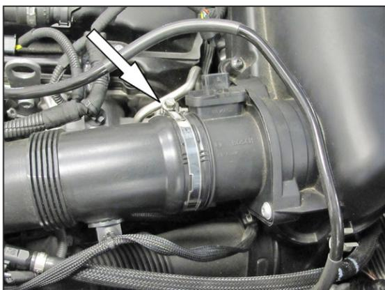
3. Loosen the hose clamp which secures the intake tube to the mass air sensor.
