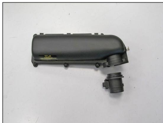
6. Remove the two screws securing the mass air sensor to the upper air box housing and then remove the sensor as shown.
