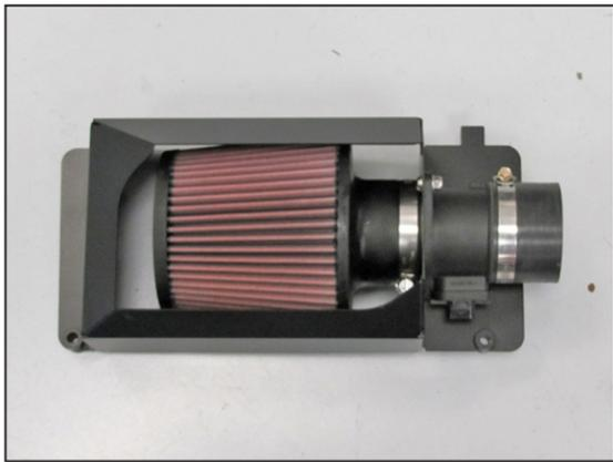
10. Install the provided silicone hose (08440) onto the mass air sensor and secure with the provided hose clamp.
