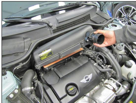
5. Remove the upper air box housing and air filter from the vehicle.
