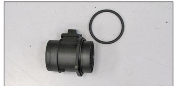
7. Remove the factory O ring from the mass air sensor.
