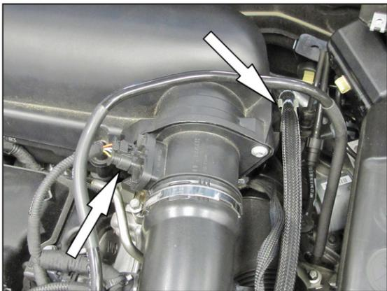
2. Disconnect the mass air sensor electrical connection and unhook the vent line from the air box.
