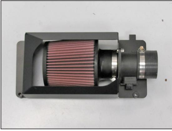
10. Install the provided silicone hose (08440) onto the mass air sensor and secure with the provided hose clamp.
