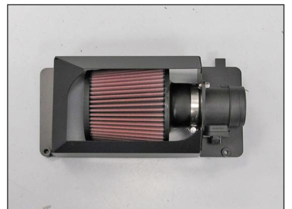
9. Install the K&N® air filter onto the mass air sensor inside the heat shield and secure with the provided hose clamp.
