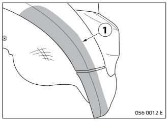
Clean gluing surfaces extensively (1).
