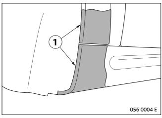
Clean gluing surfaces extensively (1).
