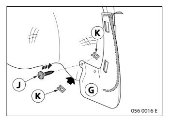
Screw self-tapping screw **J** into the existing hole of mud flap **G** and through the wheel arch trim. Brace when bolting sheet metal nut **K** to the back of the wheel arch trim.
