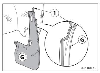
Undo approx. 2-3 cm protective film (1) off the gluing pads of mud flap  ${\bf G}$ .
