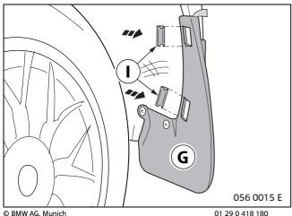
Affix mud flap **G** with metal tabs **I** on the wheel arch seam.
