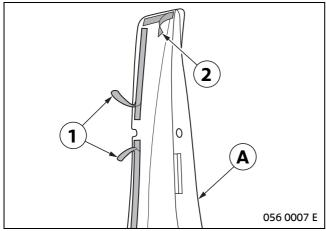
Pull approx. 2-3 cm. protective film (1) off the gluing pads from each mud flap **A**.
