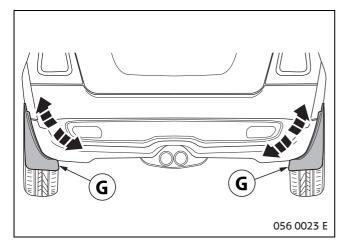
Fit the wheels on the vehicle and allow the vehicle to settle completely on the ground. Align mud flaps **G** evenly.
