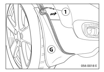
Pull protective film (1) completely off the gluing pads and press on mud flap **G** with a force of approx. 5 kg.
