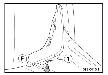
Insert dowel **F** into the bore (1) from the underside of the vehicle.
