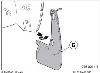
Position mud flap **G** on the vehicle from below and put into place.
