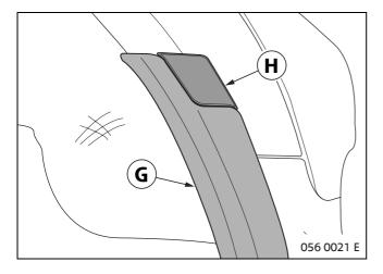
Insert cover **H** precisely in the recess of mud flap **G** and press on with a force of approx. 5 kg.
