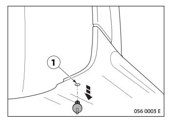
In the rear left wheel arch, pull out expander rivet (1). It is no longer required.
