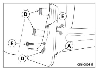
Position mud flap **A** precisely on the vehicle and attach to the vehicle with metal tabs **D**.
