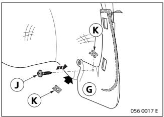
Bolt second self-tapping screw **J** into the existing hole of mud flap **G** and through the wheel arch trim. Brace when bolting sheet metal nut **K** to the back of the wheel arch trim.
