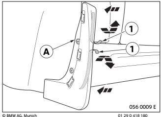
Pull protective film (1) completely off the gluing pads and press on mud flap **A** with a force of approx. 5 kg.
