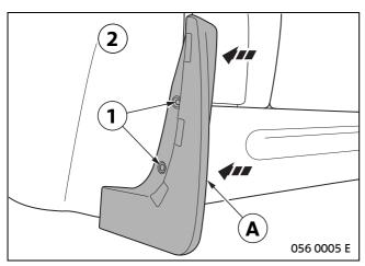
Position mud flaps **A** precisely and transfer bores (1) onto wheel arch cover (2).
