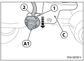
Fit branch A1 in socket bracket C.
