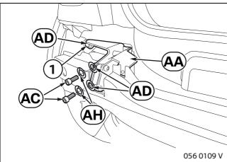
Install left mount **AA** and secure at top left with original screw (1) as well as screws **AC**, washers **AD** a retaining rings **AH**.
