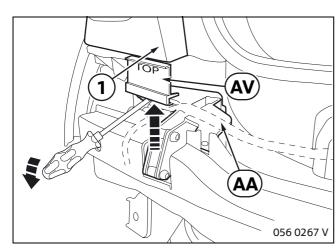
Use a screwdriver to lever up left mount **AA** while screwing down so that the spacing gauge **AV** is clamped free of play between mount **AA** and rear light base (1). Tighten all screws of mount **AA** and of the bumper to 21 Nm.
