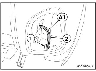
Working from the inside, pass branch A1 through hole (1) to the outside.
