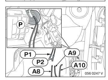
In the vehicle interior, pull cable **P** through the rubber grommet. Seal off the rubber grommet.
