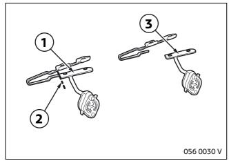
Separate the exhaust bracket (1) at edge (2). Only the separated piece (3) is used for installing the socket bracket **C**.
