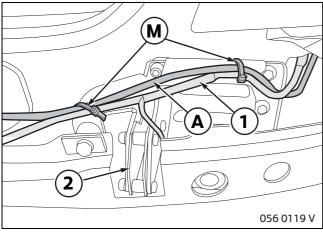
If necessary, secure wiring loom **A** together with **t**he cable for the rear fog lights (1) with cable strap **M** to rear rack mount **AB**.
