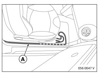
Route wiring loom **A** along the sill to the fuse panel in the passenger's footwell.
