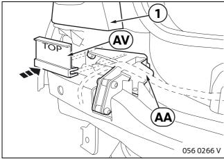
Fit spacing gauge **AV** on left mount **AA**.
