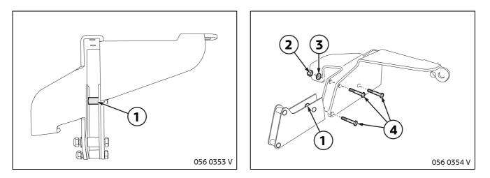
Check bush (1) before starting the work on the two rear rack mounts. If **creme-coloured plastic bushes** (1) are fitted, they must be replaced. For this purpose, order the repair kit, **Part No. 82 71 0 418 155**, and proceed as follows:
