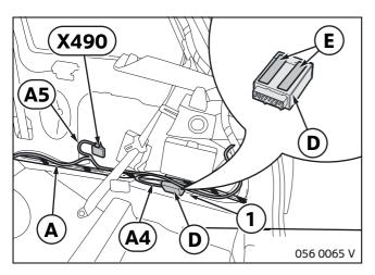
Cut Velcro strip **E** in two equal lengths. Peel protective strips from adhesive surfaces and adhere next to each other on the underside of the control unit **D**.
