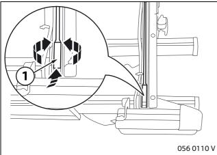
Carefully lift the sliding block (1) out of the guide.
