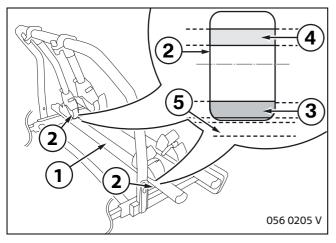
If there is play in the aluminium rear rack, first visually check the bushes in the mount assemblies under the rear apron. **Creme-coloured plastic bushes** (1) may be fitted which are broken or damaged. If damaged, the plastic bushes (1) must be replaced in pairs by bronze-coloured metal bushes.
