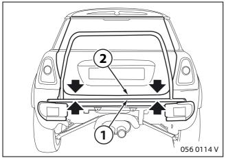
At this point continue with section 11, Checking adjustment of aluminium rear rack. •
