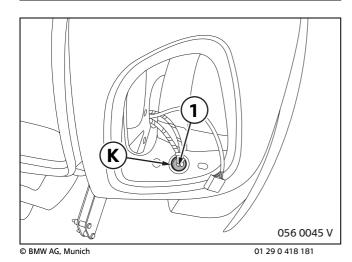
Fit grommet **K** in the hole. Pack the grommet with Betalink adhesive (1).
