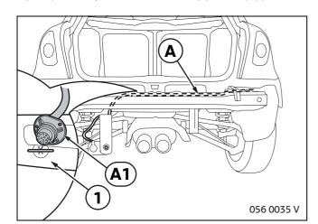
Route wiring loom **A** to the left at the top of the bumper. Pass branch **A1** through the foam material moulding (1).
