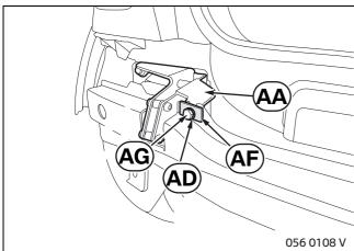
Secure shim **AF** and washer **AD** with screw **AG** through opening (1) to mount AA. Tighten screw AG to 15 Nm.
