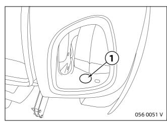
Drill out hole (1) to 40 mm Ø, deburr cut edge and protect from corrosion with zinc dust paint and primer. Follow the instructions for using the zinc dust paint.
