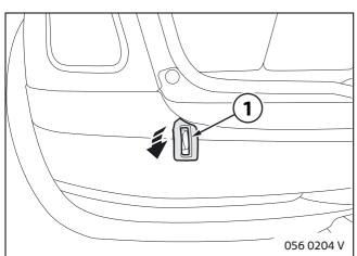
Fit trim cover (1). If necessary rework the cutouts in the rear bumper panel so that the trim cover is flush with the mount.
