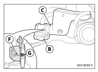
When swivelled upward, it must be possible to open the socket outlet **B** to the right. ∢
