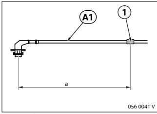
Mark the position of the grommet with adhesive tape (1) on branch **A1**:
