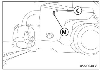
Secure cable with cable strap **M** to socket bracket **C** through the existing holes.
