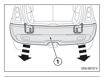
Remove rear bumper panel (1) together with the templates as described under TIS No. 51 12 156.
