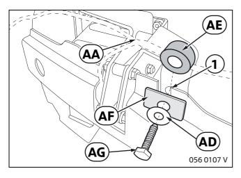
Install spacer bush **AE** between mount **AA** and the crash beam.
