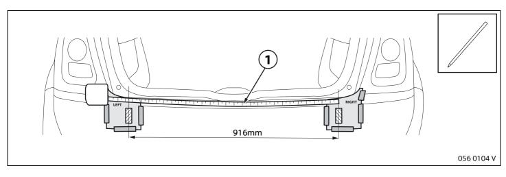
Use a tape measure (1) to transfer the distance between the centres of the templates (= 916 mm, see table on page 7) on to the left-hand side. The distance between centres must be measured along the outer contour of the rear bumper panel.
