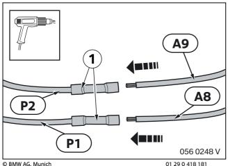
Using connector (1), crimp the insulated branches A8 (RTVI) and A9 (RTWS) of the rear rack wiring loom A with the branches P1 and P2 of the retrofit battery wiring loom P.
