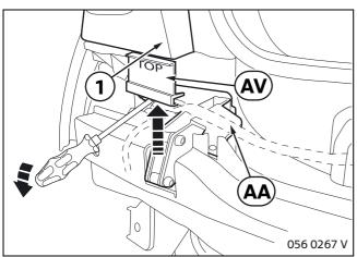
Use a screwdriver to lever up left mount **AA** while screwing down so that the spacing gauge **AV** is clamped free of play between mount **AA** and rear light base (1).
