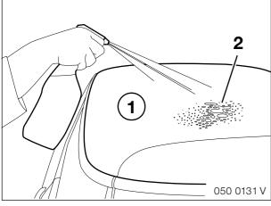
Spray the complete roof (1) with plenty of the installation solution (2).
