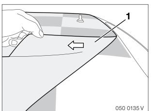
Ensure that the foil segments are affixed to the roof and do not move. ◀
