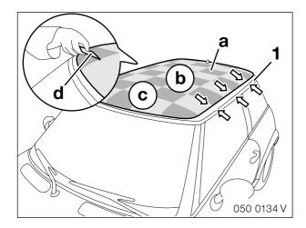
Push the three support elements **a**, **b** and **c** together until they are flush. Align the support elements to the centre of the roof by measuring the distance to the gutters (1) on each side.
