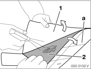
The foil segments are affixed to support elements. The adhesive side of the segments is covered with a printed backing foil.
