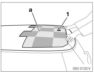
Place the support element **a** with the foil segments on the underside on the rear section of the roof. Align the support element to the aerial mounting (1).
