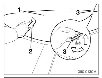
Clean the roof (1) with a cleaning cloth (2) and suitable cleaning products. The roof must then be absolutely dry, clean and free of wax and grease.
