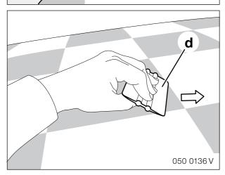
Spray the segments with installation solution at regular intervals. This makes it easier to flatten them and also prevents damaging the foil and the roof paintwork.
