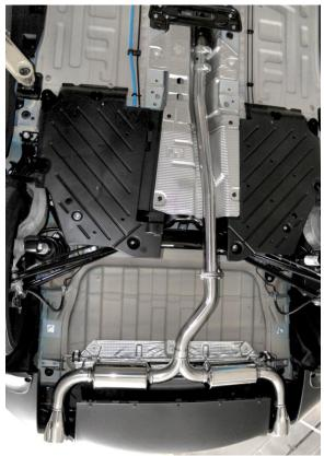
Double check complete installation. Clean exhaust with contact cleaner before starting so no oil marks burn into stainless steel.
