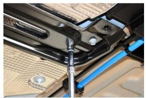
Remove exhaust tunnel cross-brace, (4) 10MM Hex Bolts.
