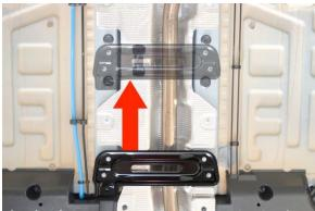
Re-install cross tunnel brace. NOTE: Front wheel drive only; if brace touches exhaust pipe then move brace to forward holes as pictured. The factory self tapping bolts will cut threads into the blank holes.
