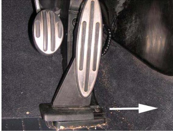
8. Carefully arrange the Sprint Booster module behind the accelerator as you re-install the accelerator module. Slide the entire module back in place while making sure the Spring Booster module does not bind against anything. Once the module ‘snaps’ into place, it’s done!
