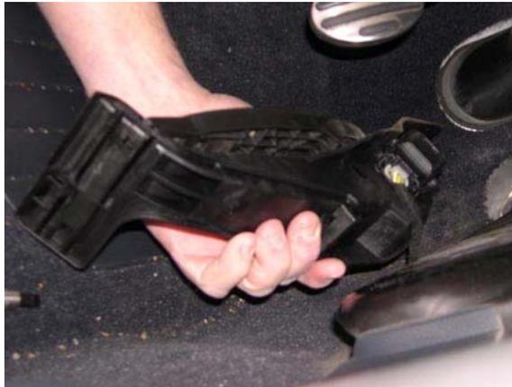
4. Flip the accelerator module on its side to expose the electrical connector. There are latches that need to be 'released' in order for the connector to unplug. While holding the module with one hand, squeeze the connector on the sides with your other hand (squeezing the latches) as you pull it free. It's a little tight, but it will come free.
