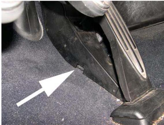
2. Image below shows the accelerator module sliding left after the tab is released. After sliding a short distance to the left, the entire module will lift off.
