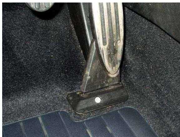
3. Using a 5mm allen wrench, remove the screw. (Torx wrench for newer models.)
