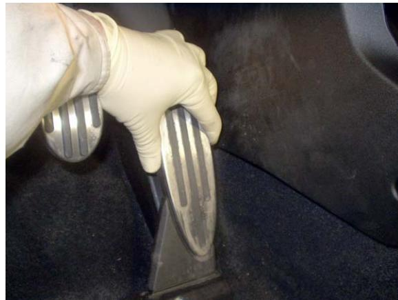
5. Flip the accelerator module on its side to expose the electrical connector. There are latches that need to be 'released' in order for the connector to unplug. While holding the module with one hand, squeeze the connector on the sides with your other hand (squeezing the latches) as you pull it free. It's a little tight, but it will come free.
