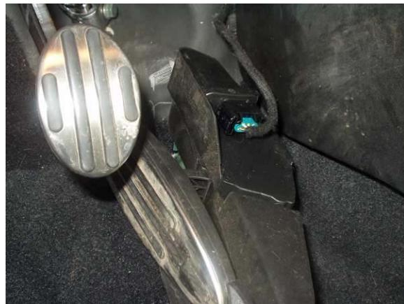
6. Get the Sprint Booster ready by plugging in the switch module – the little white connector goes into the white plug on the Sprint Booster. Much easier to do this in advance.
