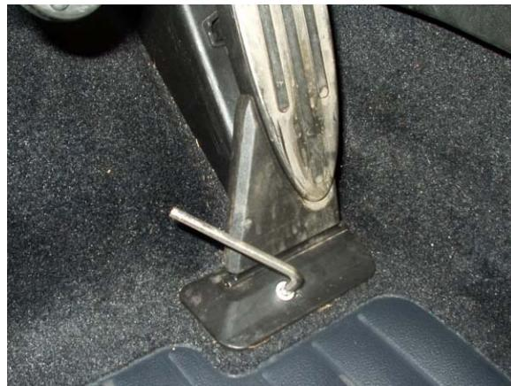
4. Lift up on the accelerator pedal module in approximately the same angle as the floorboard as it rises up to the firewall to remove the module and access the connector on the back side.
