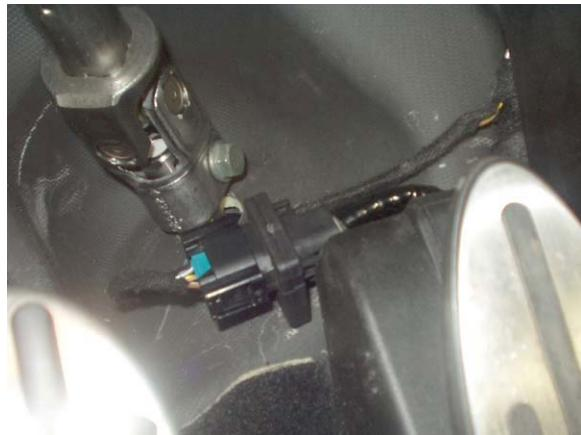
10. Route the switch module cable into the center console making sure it does NOT interfere with the pedal movement. Set the switch module in the center console, or in the cupholder for now.
