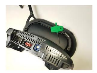
**Step 3 - Re-Install the Tachometer**
