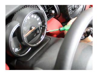
The tachometer is fastened to brackets on top of the steering column, so take note of this as you remove it. It will be important to realign the tach onto these brackets for proper reinstallation.
