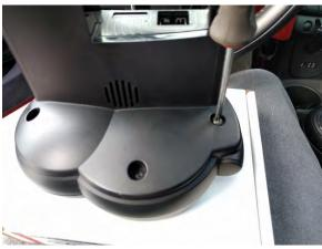
For newer Digital Clusters, use the included T8 Torx driver to remove the 4 screws holding the unit together (shown below). You will not need these to complete the installation, but it is a good idea to hang onto them in case you ever remove the Gemini Mount.
