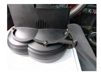
Digital Clusters have their bracket installed similarly. Align the bracket with its spacers over the four holes.
