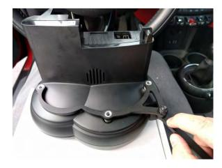
Use the included screws to secure the bracket to the back of the tach. To ensure a secure attachment of the bracket to the tach, these screws are slightly longer and wider than the factory screws. They will require a bit more torque to install than the stock screws, so once the screw bottoms out, do not keep tightening as you risk stripping the hole.
