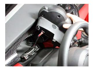
Step 2 - Install the Bracket onto the Tachometer
