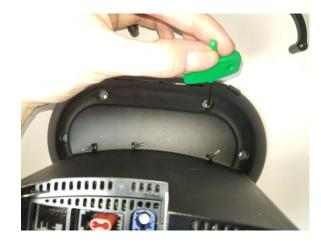
Align the bracket with its aluminum spacers over the three holes.
