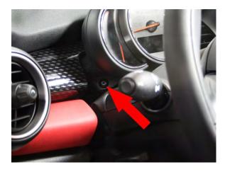
Find the 2 Torx screws that fasten the tachometer to the steering column and remove them using the T-20 Torx driver. They may be covered with rubber caps. Be careful not to drop them as this can double your install time! (This is where a magnetic tip comes in handy) Keep these Torx screws safe as you will need to re-install them later.
