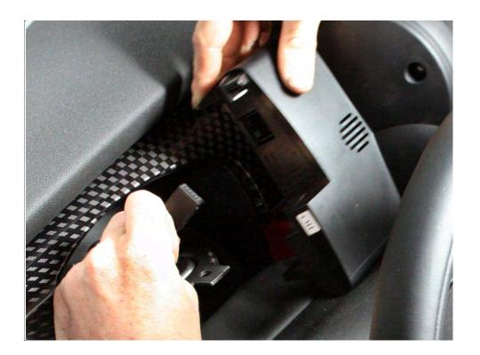
3. Remove the 3 phillips screws on the back of the housing.
