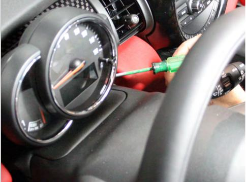
2. Pull the gauge cluster towards you and depress the lock-tab to remove the electrical plug from the rear of the unit.
