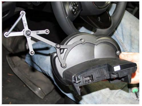
5. Re-connect the gauge cluster wiring plug, slide the unit back into place, and replace the screws on either side of the base. Don't forget the caps if you still have them!
