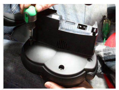
4. Place the "U" bracket in place and tighten it down using the provided screws. (Note: These screws are slightly thicker than the OEM screws) Once the bracket is secure (no wiggle), do not over-tighten as this will just strip out the plastic housing.
