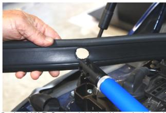
7. Install NM Tie-Bar through hole in rubber engine bay seal. Repeat for other side.
