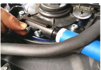
8. Attach NM Tie-Bar clevis to mounting base plates using [4] M8x20mm hex socket bolts supplied and install rubber engine bay seal at the same time.
