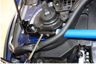
9. Tighten all [4] M8x20mm hex socket bolts using 6mm hex key wrench.
