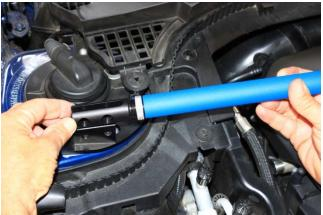
Adjust billet-end clevis holes to match-up to base plate holes.
