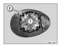
Retaining lugs (1) must not be damaged.
