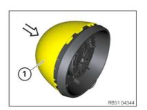
Install the protective cap (1) and engage it on all the latch mechanisms through pressure.
