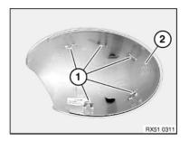
Latch mechanisms (1) on housing (2) must not be damaged.
