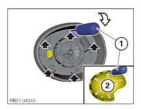
Unlock the protective cap using a small screwdriver (1) through the bore holes (see arrows). Unlock the protective cap with a slight tug clockwise on the retaining lugs (2).
