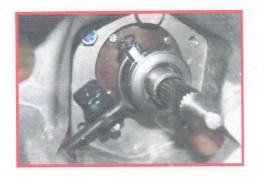
(*Note:* check the pivot bolt & the bearing in the clutch fork for wear as this may impair the clutch travel and operation.) Tighten to remove side play but do not impair lever action. (See notes on clutch release bearing).
