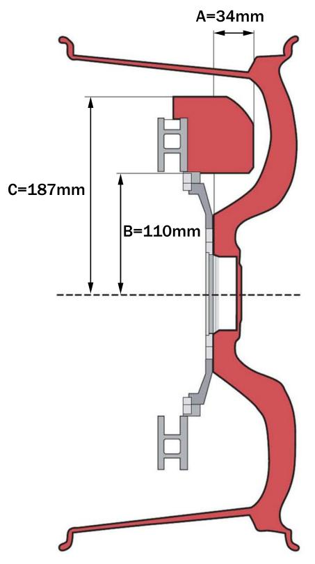
NOTE: A MINIMUM OF 2.0mm CLEARANCE MUST BE MAINTAINED BETWEEN THE WHEEL AND CALIPER IN ALL AREAS
